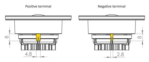
Thickness, both terminals: 0.5 mm Terminal plating: Gold
